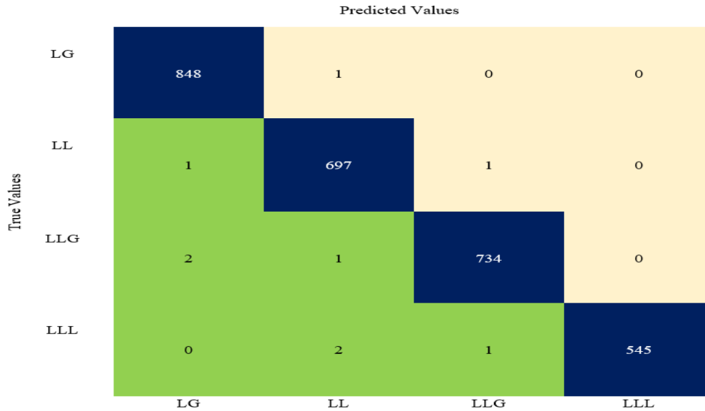
Figure 10: Confusion Matrix for fault classification using CNN model in 330kV network
